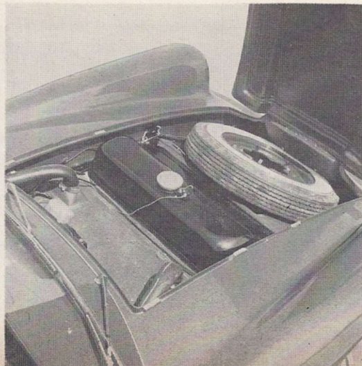
The plunging nose gives no room around the spare and tank.
